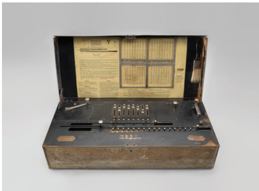
Millionaire calculating machine c. 1904 Otto Steigler (1858–1923) Hans W. Egli Zurich Courtesy of Cliff Stoll L2021.0902.012
